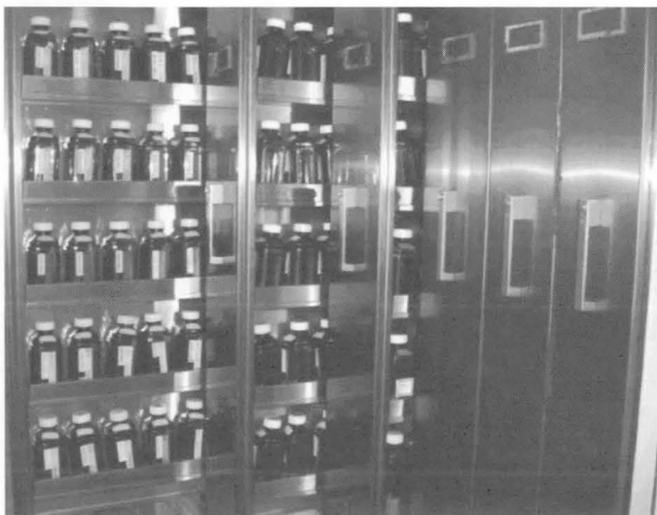
図2 水専用引き出し式冷蔵庫 Figure 2 Water exclusive use drawable type refrigerator.
